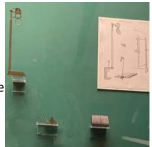
Camera Lucida,—basically a lens and mirror on a stick. It enables the artist to position the eyes nose and mouth accurately, necessary to achieve a good likeness.
